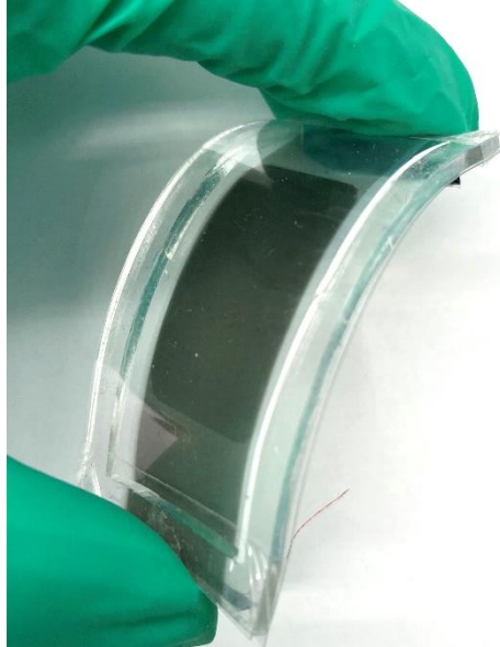
Fig. S4. The photograph of the flexible EC thermoregulation device.
